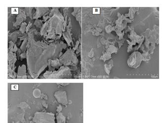
Figure 2. Scanning electron micrographs (SEM, ×3000). A: epicarp powder; B: flesh powder; C: pitted sample powder
